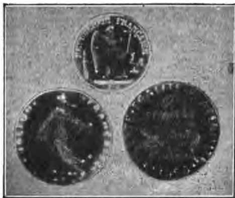
FIG. 27.—Impressions produced by ions issuing from an electrified point through a sheet of black paper.
