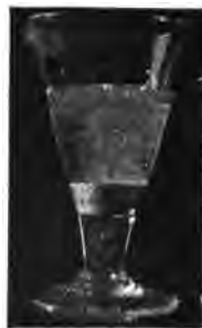
FIG. 55.— Decomposition of water by mercury containing a trace of magnesium. (Instantaneous photograph.)
