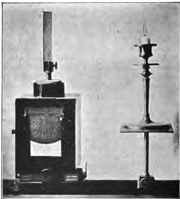
FIG. 47.—Apparatus for showing the leak of electricity under the influence of flames according to the distance and the nature of the body on which the action is produced. The charged strip on the electroscope draws to itself the ions of contrary sign which discharge it.
